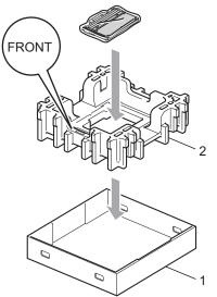
Wrap the machine with a plastic bag. Put the machine on the Styrofoam piece (1).
